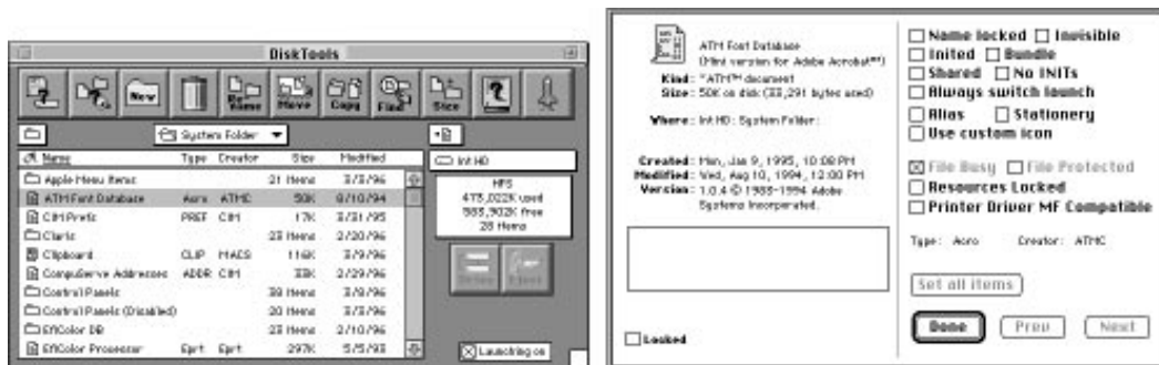
DiskTools' main window (left) and the Info window it provides for an item (right), in which you can view and manipulate a file's attributes.
